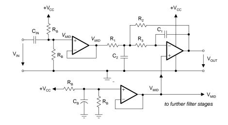
Figure 16-49. Biasing a Second-Order MFB Low-Pass Filter
