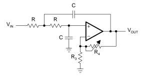
Figure 16–18. Adjustable Second-Order Low-Pass Filter
