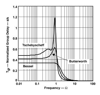
Figure 16-8. Comparison of Normalized Group Delay (Tgr) of Fourth-Order Low-Pass Filters
